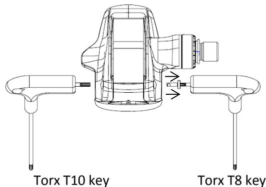
**4** Then, push with the T10 key to remove the screw inside (shouldered pin)
