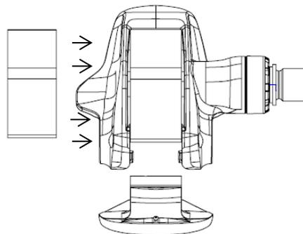
**8** Position the small silver guide supplied with the blade kit in the hollow part of the lever pin.
