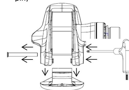
The lever and the blade are no longer attached to the pedal body now
