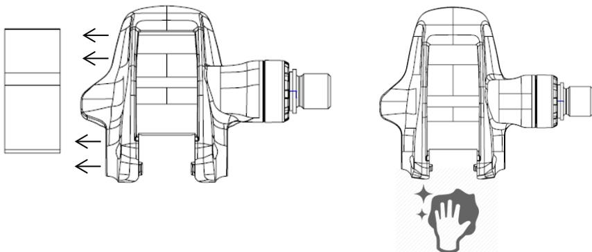
**7** Position the new blade in its seat with the tension marking towards the lever. Then, position the lever in the body pedal.
