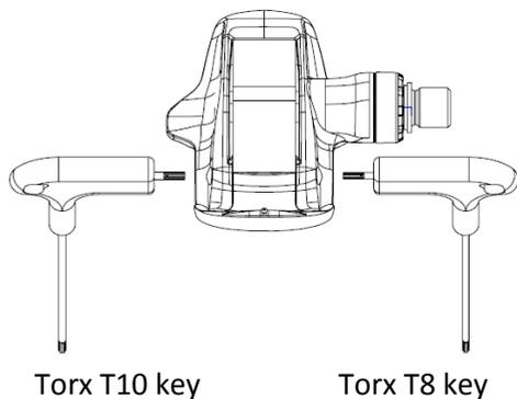
**3** Unscrew on the left while maintaining to the right with a T10 key
