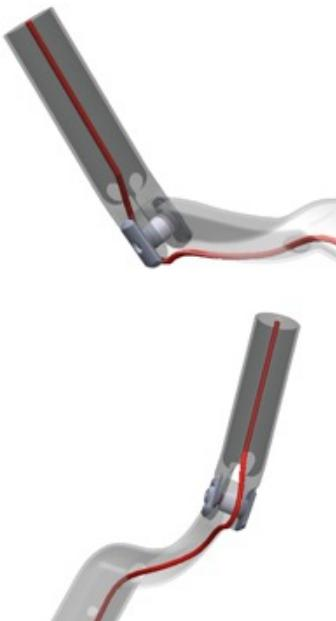
15.3 - Place the e-tube in the V (6) that supports the extension bars and add the cover only once you have routed both bars.
