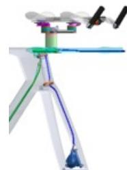
9 - Insert the front brake hose through the left fork leg and exit through the top of the head tube (dark blue hose).
