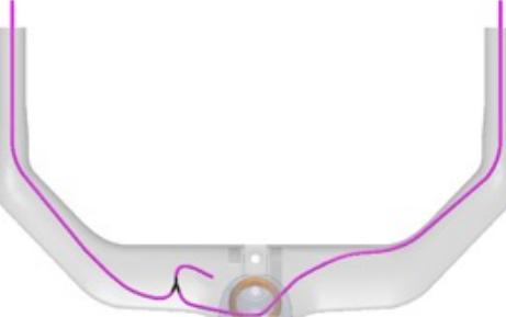
10 - Slide a pre-prepared, 510mm foam tube onto the rear brake hose.
