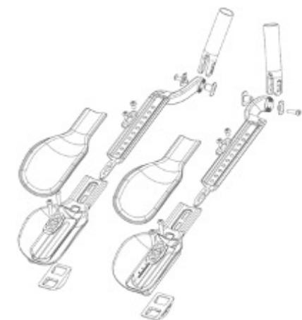
5 - Position the upper plate according to the required position and tighten the screws to a torque of 8Nm.
