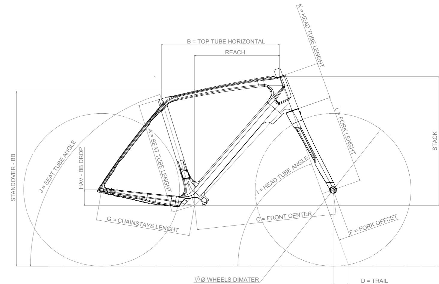
**E-765 GOTHAM GEOMETRY**      WHEELS DIAMETER IN MM : 700
