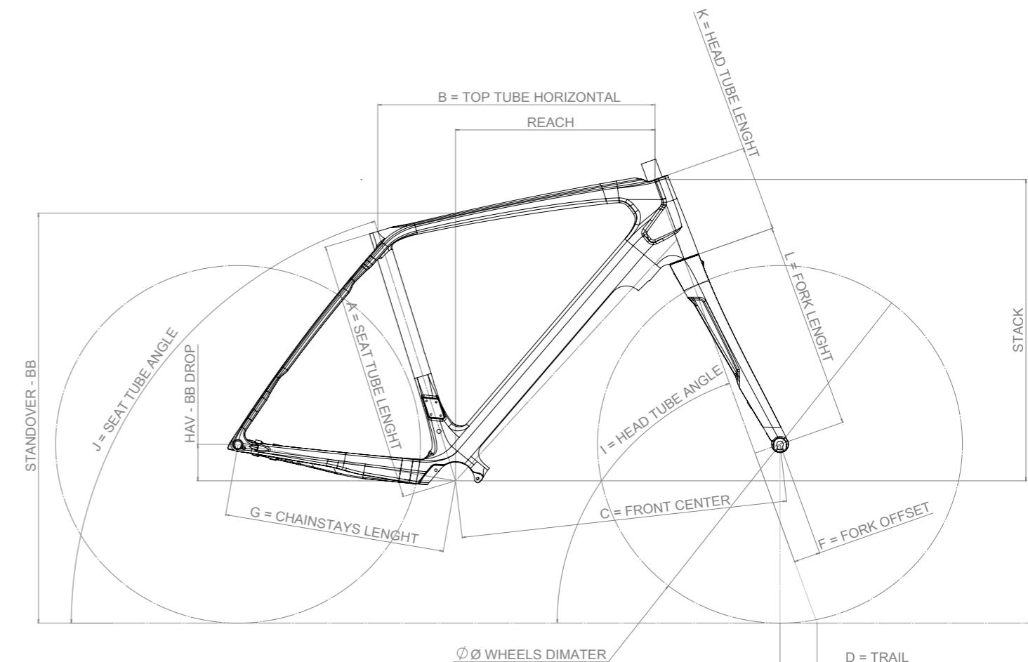
**E-765 GRAVEL GEOMETRY** WHEELS DIAMETER IN MM : 700
