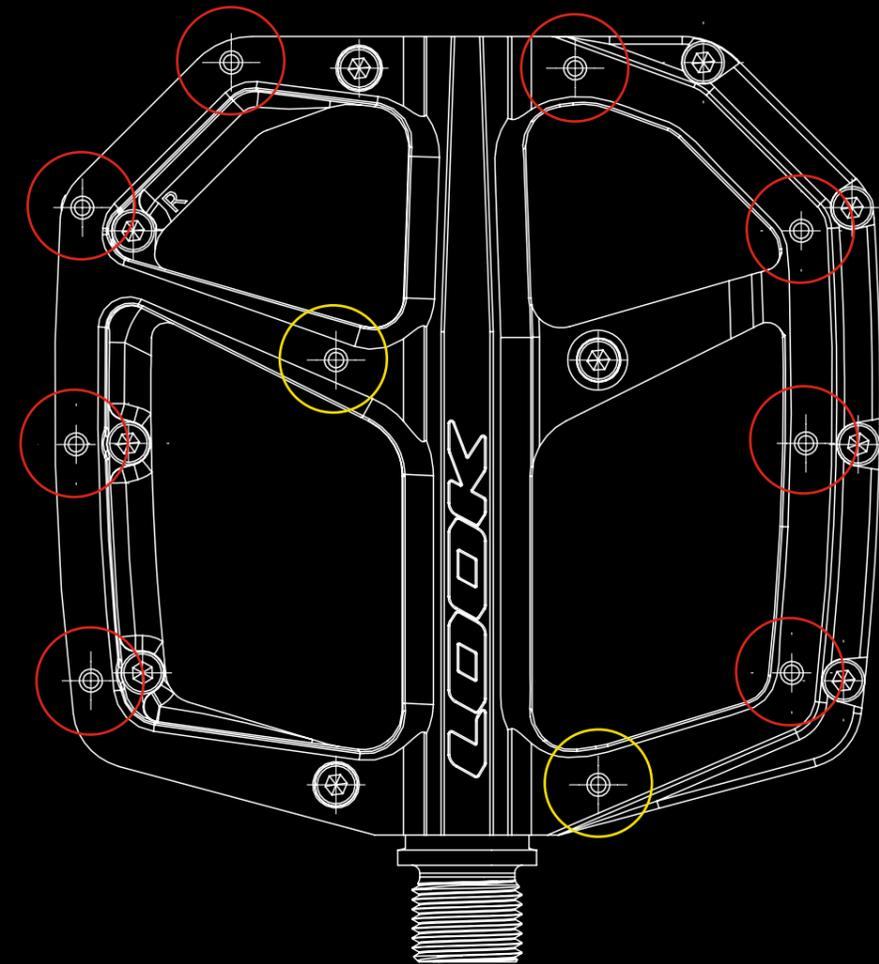
**+** Concave body shape + pins length to secure foothold
