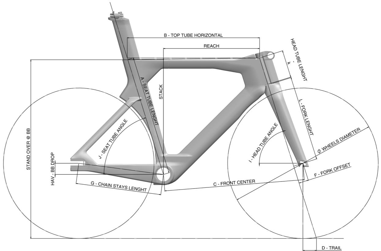
**T20 GEOMETRY** WHEEL DIAMETER IN MM : 676
