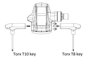
Then, push with the T10 key to remove the screw inside (shouldered pin)
