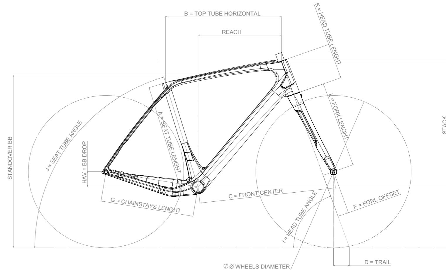
**765 GRAVEL GEOMETRY** WHEELS DIAMETER IN MM : 700
